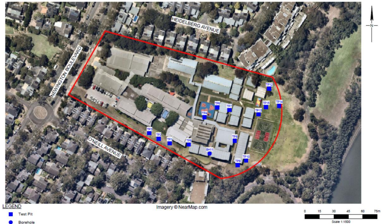
Figure 4 Locations of Test Pits and Boreholes for Preparation of Reference 7
